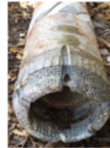
Surface-set Diamond, Stepped-Profile (HQ-size)
